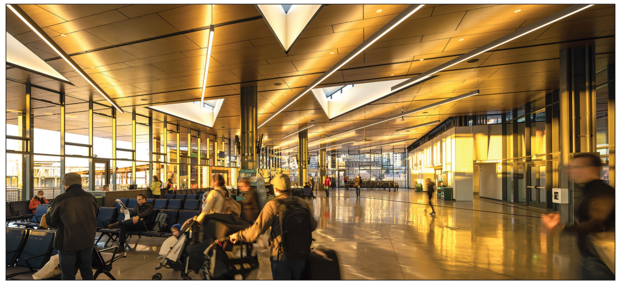
Triangular-shaped skylights bathe the waiting room with natural light, reducing the demand for artificial lighting.
